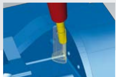
5-axis corner rest machining for efficient corner machining
