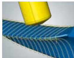
Top milling with barrel cutters
