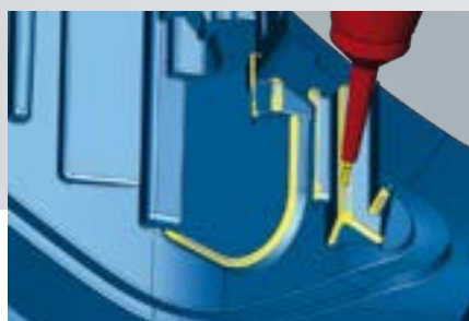
3D-automated rest machining for homogeneous toolpaths
