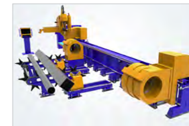
Automatic loading, feeding and unloading
