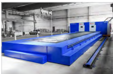
Heavy-duty fiber laser cutting machine
