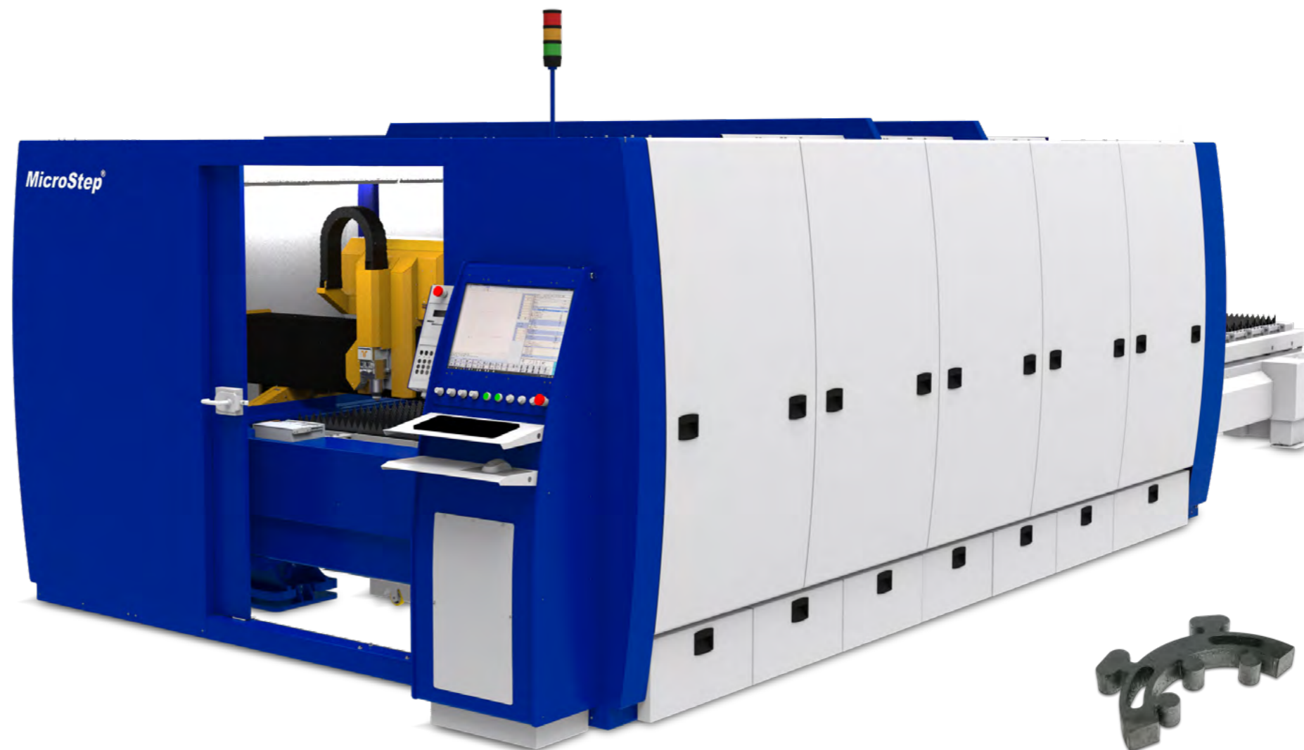
Automatic shuttle table with sectional fume extraction
