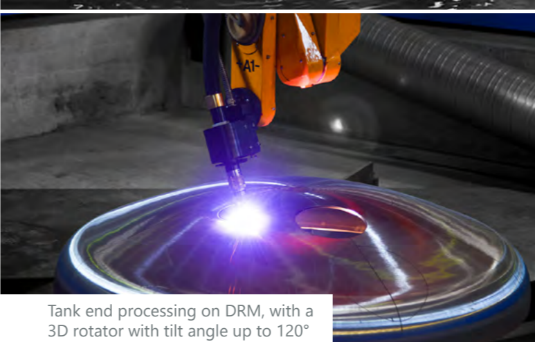
DRM machine with work area 50 x 8 meters and a water table for underwater plasma cutting
