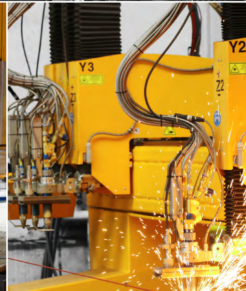
Integration of up to 8 oxyfuel tool stations on one gantry
