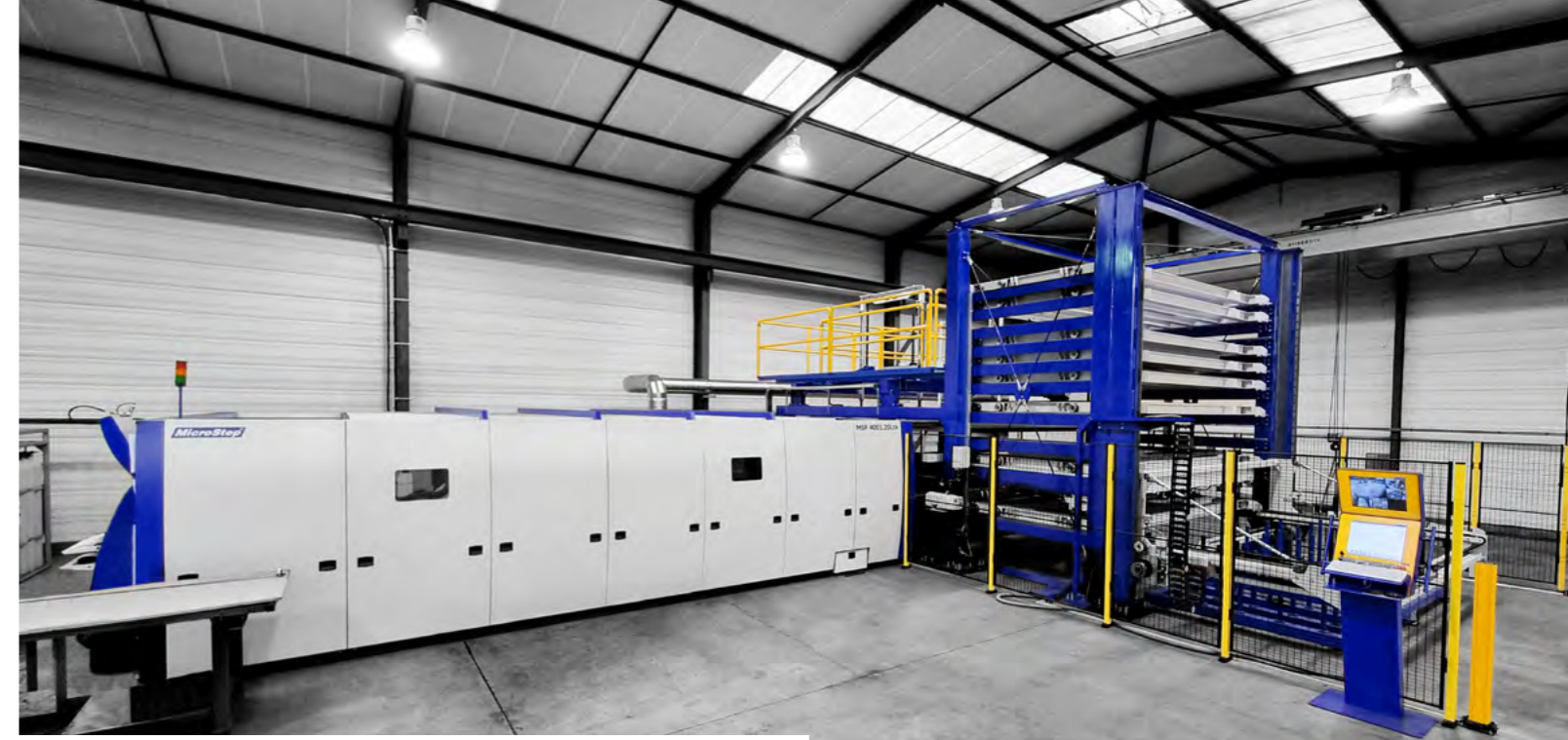
MSF Pro machines can be fully automated via material handling and sorting systems and CyberFab® Manager software
