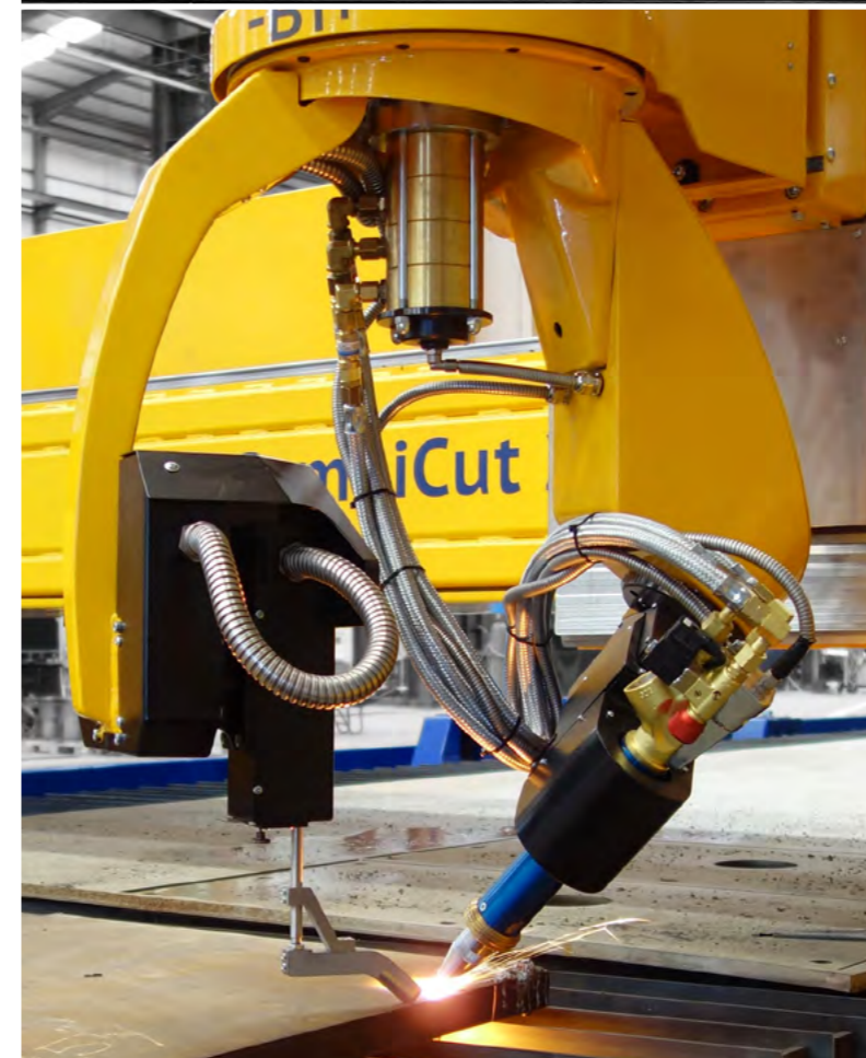
Bevel cutting with oxyfuel rotator
