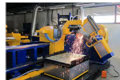
ElbowCut: Weld edge preparation on pipe elbows
